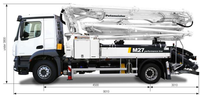
Note: Standard version. Dimensions and weights can be changed depending on vehicle, pump and equipment. Dimensions in mm, exemplary for MB Arocs 1835. Illustrations include optional extras.
